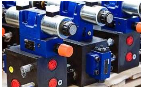
Valve Control Blocks
