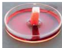
Incubating Powerbone Stick in red ink solution. Images captured in every 5 seconds. After 20 seconds sticks are completely covered.
