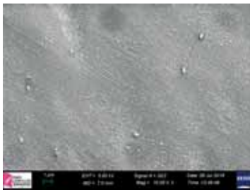
Exterieur side of Powerbone Dental Barrier Membrane compose of non-porous poly(lactic acid) (PLA) based film to prevent epitheriel cells and fibroblast migratio
