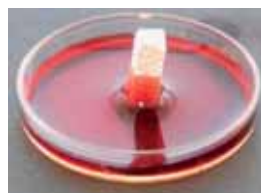
Incubating Powerbone Stick in red ink solution. Images captured in every 5 seconds. After 20 seconds sticks are completely covered.
