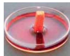
Incubating Powerbone Stick in red ink solution. Images captured in every 5 seconds. After 20 seconds sticks are completely covered.
