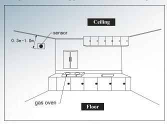
LDG detector: install the sensor at 0.3-1m above the Door, and also near the leaking gas within 1.5m(see below map)
