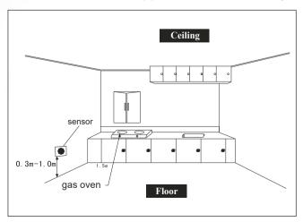
2. Hang the detector on the wall,make sure it is stable and xed. 3. when installing the sensor for home use, do not install in dirty, dusty or oily areas, such as the kitchen House, garage and house. Oil, dust, or household chemicals can contaminate sensor head, so that alarm can not working properly. Do not block the ventilation opening. The Detector will not be installed by curtains, furniture or other objects blocking the air
