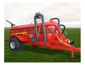
Liquid manure spreader is designed to suck the slurry from the pool and spread to the land homogeneously.
