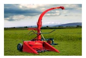
"The Row Independent Maize Chopper has a working width of 1,25m. and with its cutter and feeder drum it can chop two rows of maize at one pass. One of the most important specification of the machine is its foldable chassis. The chassis can be folded so that the machine stays behind of the tractor. By driving backwards the machine can open a way in the middle of the field in order to decrease the number of turns on the field and decrease the fuel consumption of tractor.
