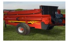
"Manure spreader is designed for spreading the manure on the fields, garden and orchard. The chain conveyor carries the manure to the beater at the back of the machine and the manure is spread on the field homogenously. The low height of the machine is advantage for the orchard and vineyards. It is trailed without damaging the trees and grapes. The floor is made of plywood to provide a long life usage. The 4 speed strong gearbox and the strong chain provides an operation without trouble.
