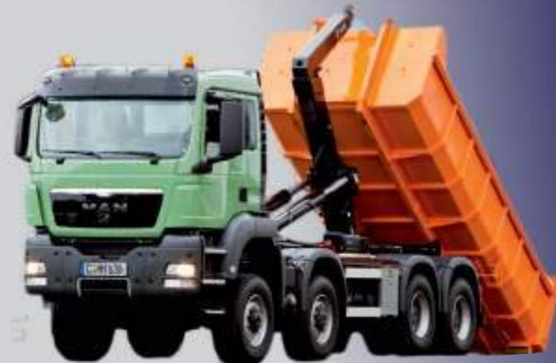
Hooklift is used to load specially manufactured wheeled containers (DIN30722) and unload to the desired spot. The platformed system acts as a damper and helps to unload the material in the container. Equipment consists of 1 lifting arm, chassis and hydraulic system.
