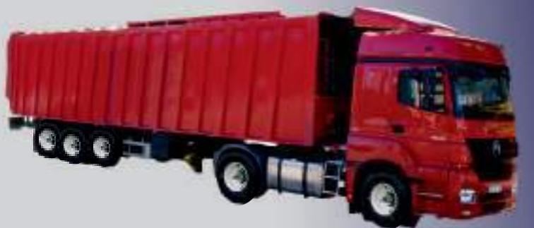
Garbage semi-trailers are used for transporting garbage to waste disposal sites. The garbage that collected by compactors are transferred to semi-trailers via unloading stations, which makes whole unloading operation easier and economical.
