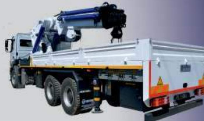
Cranes mounted between the cabin behind the vehicle and the car cabin are produced in desired tonnages in direction of demand. The weights lifted by the crane are placed on the case and transported to the desired position. The crane is equipped with 2 support legs and has 360 degree rotation capacity. When not in use, it breaks and folds and takes up little space in the car and is also suitable for use as a transport vehicle.
