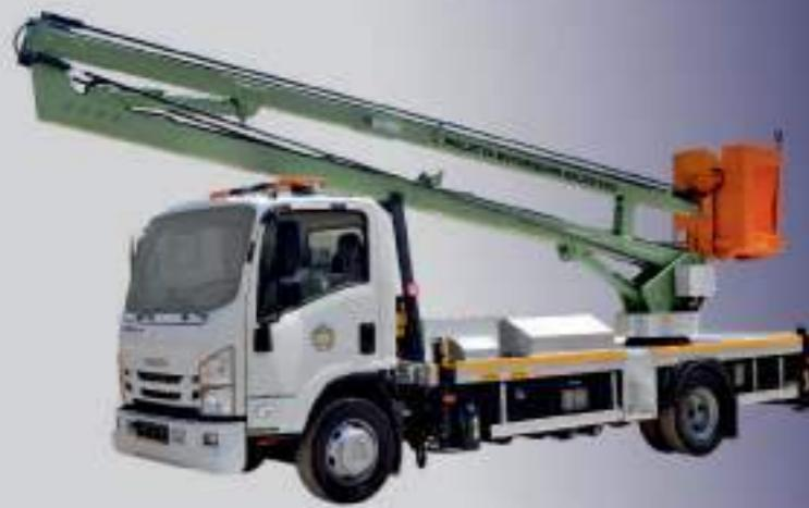
Telescopic platforms / booms are used for external cleaning of buildings, maintenance and repair of electricity lines, construction sites, pruning of high trees etc.
