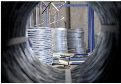
Material: Low-carbon steel wire Coating: Hot-dip galvanized (Zn) Wire Diameter: 1.50 - 5.00 mm Volume of Coating: 40 - 300 g/m<sup>2</sup> Tensile Strength: 350 - 900 N/mm<sup>2</sup>
