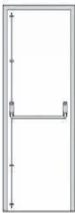
Single Door With Panic Bolt Fitted
