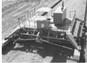
Beton Finiřeri Concrete Finisher
