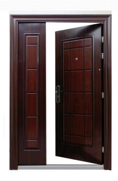
door leaf plate: 1.2mm metal, door frame sheet: 2mm metal, door frame jamb plate: 1.5mm inner and outer mdf: 8mm safety pin: 6 pcs hinge: 3 pcs door leaf seal: german binoculars. wide angle glass lock: central (14 point locked) natural wood and PVC coatin. Glass and without glass villa door
