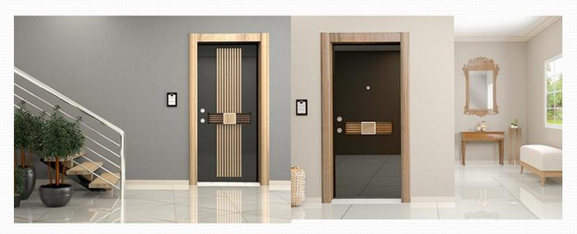
door leaf plate: 1.2mm metal dkp, door frame sheet: 2mm dkp door frame jamb plate: 1.5mm metal dkp, inner and outer mdf: 8mm safety pin: 6 pcs hinge: 3 pcs door leaf seal: german binoculars. wide angle glass lock: central (14 point locked) wood natural and black highglass
