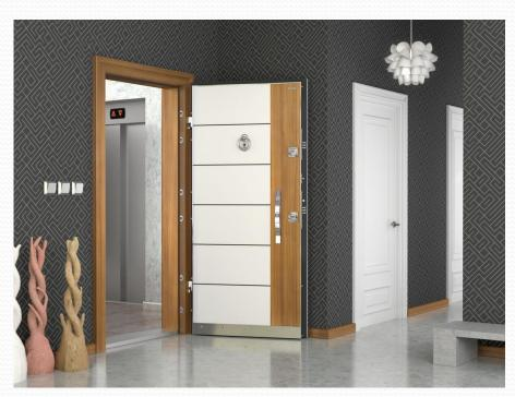
door leaf plate: 1.2mm metal dkp, door frame sheet: 2mm door frame jamb plate: 1.5mm dkp metal, inner and outer mdf: 8mm safety pin: 6 pcs hinge: 3 pcs door leaf seal: german binoculars. wide angle glass lock: mono (6 point locked)
