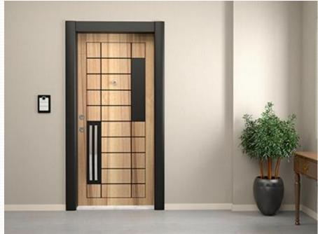
door leaf plate: 1.2mm metal dkp, door frame sheet: 2mm dkp door frame jamb plate: 1.5mm metal dkp, inner and outer mdf: 8mm safety pin: 6 pcs hinge: 3 pcs door leaf seal: german binoculars. wide angle glass lock: central (14 point locked)and mono (6 point locked) wood natural and black highglass
