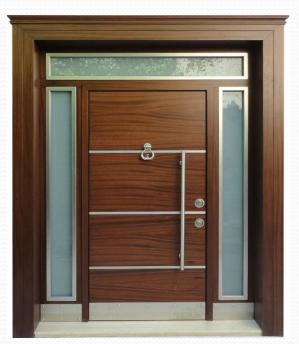
door leaf plate: 1.2mm metal, door frame sheet: 2mm metal, door frame jamb plate: 1.5mm inner and outer mdf: 8mm safety pin: 6 pcs hinge: 3 pcs door leaf seal: german binoculars. wide angle glass lock: central (14 point locked) natural wood and PVC coatin. Glass villa door
