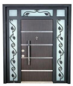
door leaf plate: 1.2mm metal dkp, door frame sheet: 2mm metal ,door frame jamb plate: 1.5mm dkp inner and outer mdf: 8mm safety pin: 6 pcs hinge: 3 pcs door leaf seal: german binoculars. wide angle glass lock: central (14 point locked) natural wood and PVC coatin. Glass villa door
