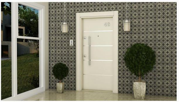
door leaf plate: 1.2mm meta dkp , door frame sheet: 2mm dkp door frame jamb plate: 1.5mm meta dkp , inner and outer mdf: 8mm safety pin: 6 pcs hinge: 3 pcs door leaf seal: german binoculars. wide angle glass lock: mono (6 point locked)
