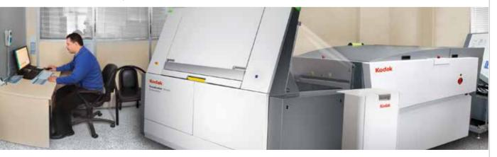
Imak Offset like many other advanced printing houses uses the direct computer-to-plate exposure. This technology ensures the minimum colour quality loss during the image transfer. This process involves CIP4 protocol that transfers technical values of the image to the control panel of the print machine and the machine performs all necessary colour adjustments automatically.
