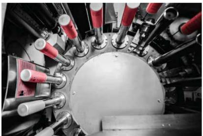
Kont Aluminyum uses advanced high-speed dry offset printing techniques up 9 colors.
