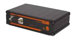
GM-1 GSM Modem, by connecting to the RS232 port of your UPS externally, provides an informative short message to be sent to the GSM numbers you specify, if alarm and operating status information is selected according to your wishes. Suitable for devices with SNMP module installed. If you do not have an SNMP module or your infrastructure does not support it, you can choose GM-2/GM-3 GSM modems in the accessories product group.
