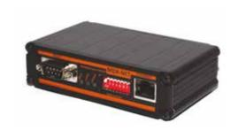
The MDX-NET RS232-MODBUS Adapter is an external MODBUS module used for UPS and STS. It converts RS232 protocol to MODBUS protocol for SCADA and BMS systems using TCP/IP Network.
