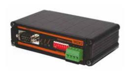
The MDX2 RS232-MODBUS Adapter is an external MODBUS module used for UPS and STS. It converts RS232 protocol to MODBUS RTU protocol for SCADA and BMS systems used RS485 Network.
