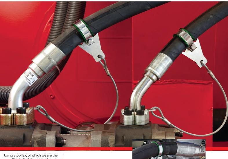
Using Stopflex, of which we are the Official Distributor, the hose is secured to the installation with a rope that protects both the operator and the components. The Stopflex system has been manufactured and tested to ensure that all hoses are held to maximum pressure.
