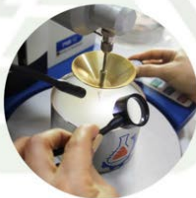
Cone Penetration test
