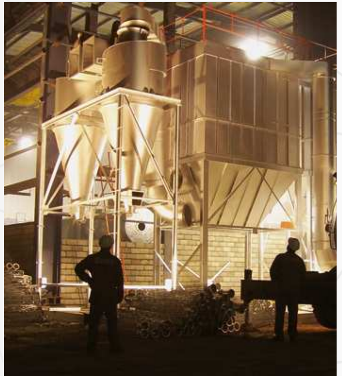
Capacity: 40.000 m 3 /h @ 450 mmWC • Motor Power: 75 kW Filtration Area: 432 m 2 • Project: Turkey • Sector: Steel Application: Dryer Filter
