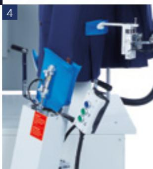
Sleeve tensioning device
