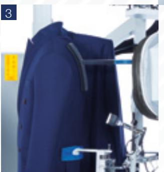
Side part tensioning device
