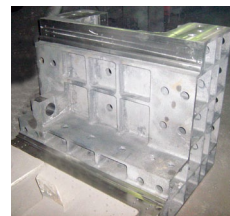
Cnc Tezgah Gövdesi (Strafor Modelden) Cnc Machine Body (Made By Foam) GG25 3.500 KG
