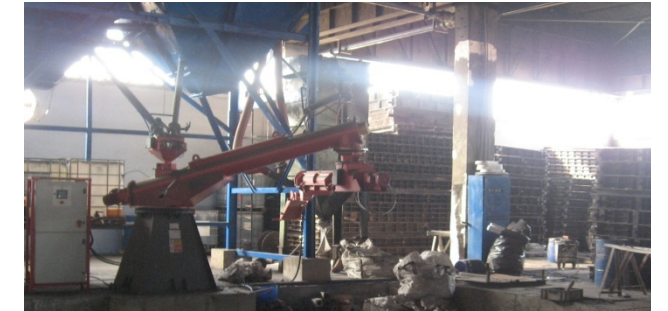
Hol Kalıplama Mikseri 10 ton/saat Hall Moulding Mixer 10 tons/hour
