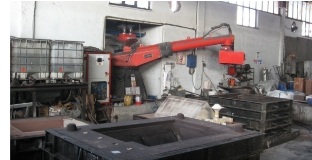
Hol Kalıplama Mikseri 20 ton/saat Hall Moulding Mixer 20 tons/hour
