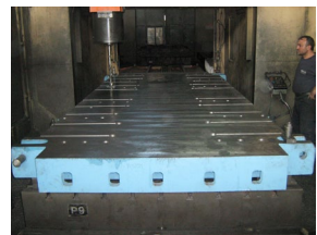
Tezgah Pleyti Batch Plate GG25 8.500 KG
