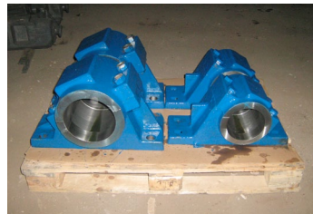
Yatak Bed Gs45 500 KG - 300 KG
