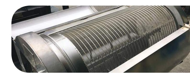
Depending on the required subtraction rate, particles from their structures or it is filtered independently of their density. The accumulated on the filter is removed particles 100% backwash efficiency it is vacuumed with. Backwashing process pressure depends on the difference. Backwashing process during filtration is continuous. Filter according to the required filter precision, the element it can be easily changed.
