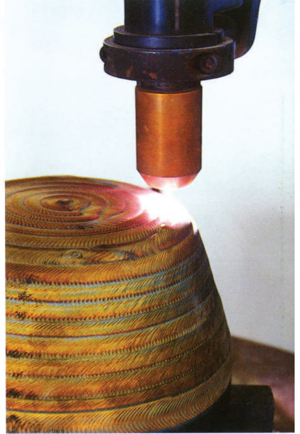
Cobalt hardfacing of a plunger by P.T.A.
