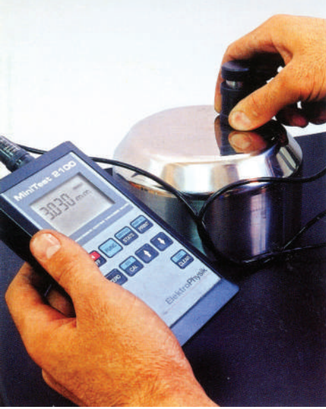
Coating thickness measurement of a borosilicate plunger
