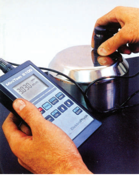
Coating thickness measurement of a borosilicate plunger
