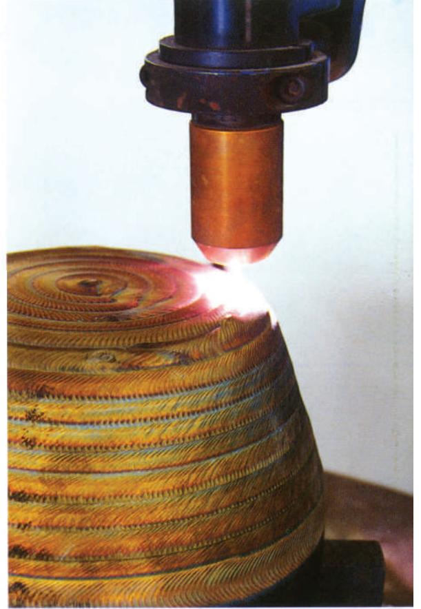
Cobalt hardfacing of a plunger by P.T.A.
