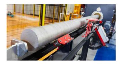
Billets are heated to the appropriate temperature value before extrusion and then passed through special molds to be brought to the desired shape. The surface quality of the billets used by Elbi Aluminium is quite high. This prevents surface from defects during the extrusion process.
