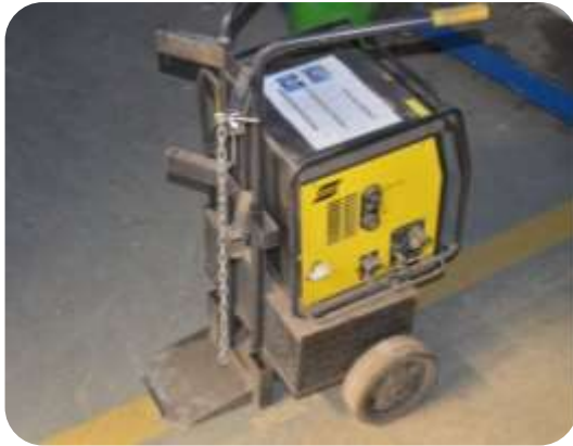
Orbital Welding Machine up to 3" t: 2mm
