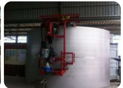
Automatic Girth Welders I: 1,000 A Ø: 5.0 m (min)
