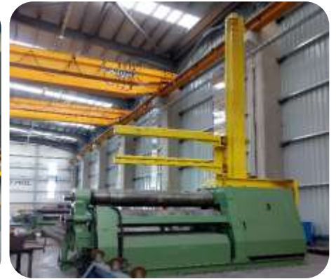
NC/CNC Rolling Machines (4 each) W: 2.5 m t: 40 mm Ø: 0.75 m
