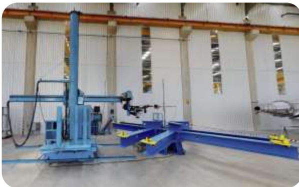
Plasma Welding Machine I: 1,000 A t: 10 mm
