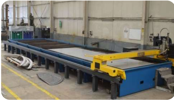
CNC Oxy-Plasma Cutting Machines (2 each) W: 3 m L:12 m max t (plasma)=55mm, max t (oxy)=150mm
