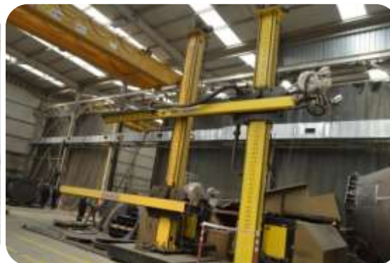
Column-Boom Submerged Arc Welding Machines (4 each) I: 1, 000 A
