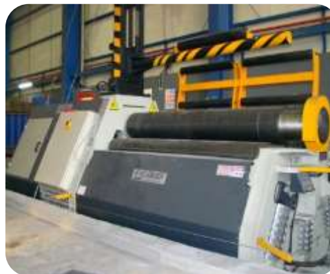
NC/CNC Rolling Machines (4 each) W: 2.5 m t: 40 mm Ø: 0.75 m
