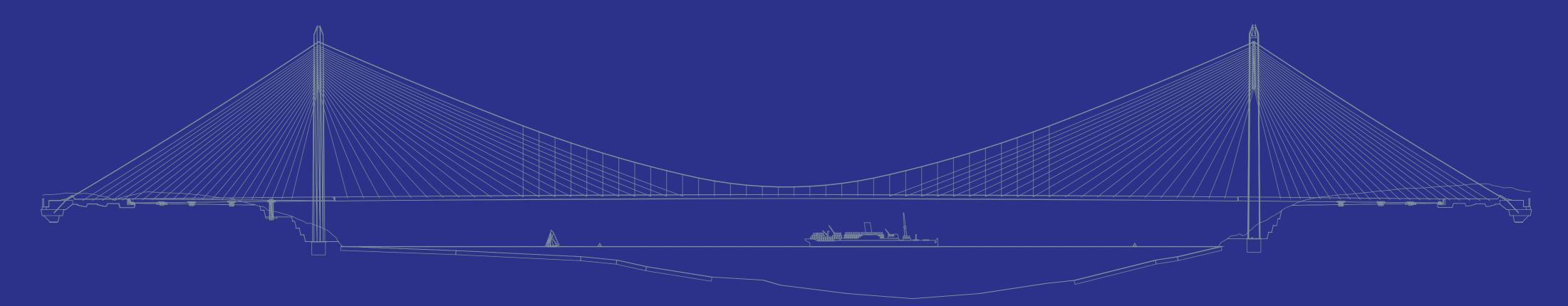
Main Span 1.408 m Total Bridge Length 2.164 m Highest Tower 322 m
