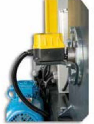
Alt Üst Limit Sivici Lower-Upper Rotation Limit Switich
