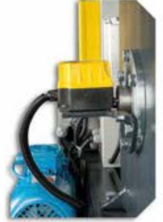
Alt Üst Tur Limit Sivici Lower-Upper Rotation Limit Switth
