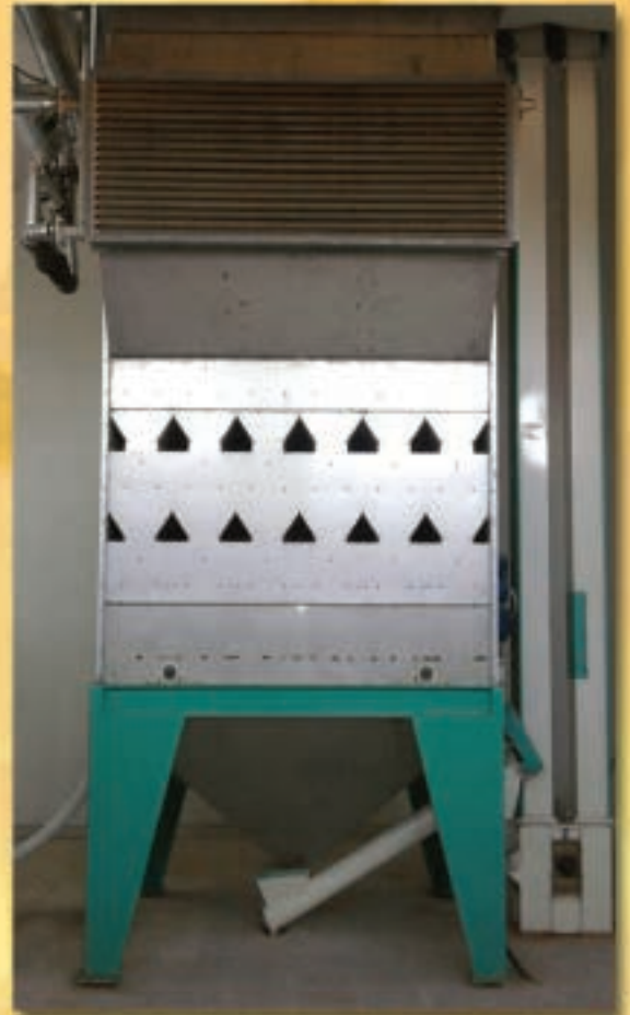
Bulgur Kurutma Kulesi / Bulgur Dryer Tower
