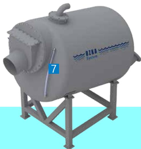
This vacuum system transfers fish safely, ensuring no harm during the process. The vacuum tank, manufactured from 316L stainless steel, features easily removable flap valves at the inlet and outlet. Additionally, the tank fills and discharges automatically using upper and lower sensors.
