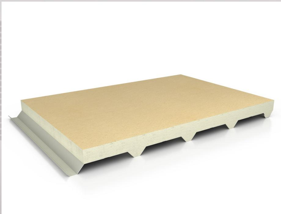
Used in poultry, farms, animal barns and etc. or used in asidic environment for their resistancy to chemicals and chemical waste. Used at the inner face of the panel. Outer face is either galvanized sheet or aliminium. The insulation material is EPS, PUR or PIR. The thickness of the pet is 0,90 mm and the thickness of the FRP is 0,80 mm.
