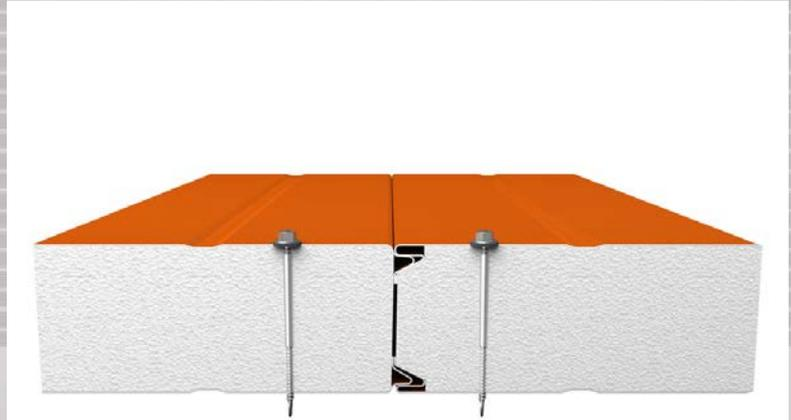
Our panel which is used in cooling, shocking and hygiene chambers and manufactured in the width of 850-1.150 mm is manufactured in different thickness and painted in line with the food regulation, thus hygiene is provided. Cold room stores provide impermeability thanks to special compound detail and shall be a solution partner for your problems.
