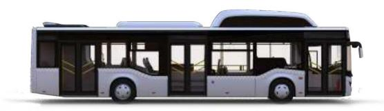
Citiport offers a green transport solution too. CNG version of Citiport 12 is available with Cummins engine which produces 320 PS and 1357 Nm torque. ZF Ecolife full automatic transmission is offered as standard. Customers may select one of two gas tank options: type 3 gas tanks with 5 units (1470 LT total volume) or type 4 gas tanks with 5 units (1175 LT total volume).
